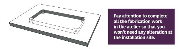
In standard sink usage, the mounting hole opened for mounting on the slab should be up to the maximum half of the slab.
