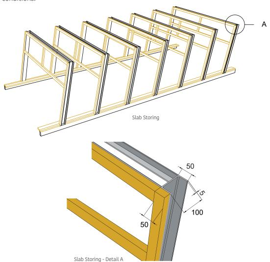
When slabs are not stored correctly, problems like warping, dirt and scratching may occur.
